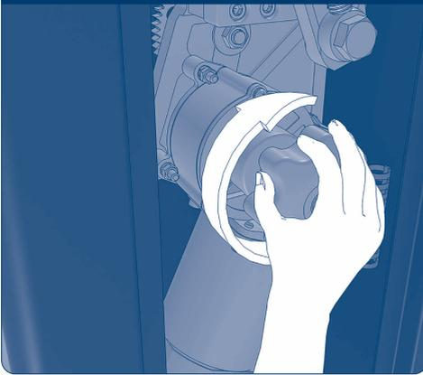
Fig. 2. Switching to automatic control mode
